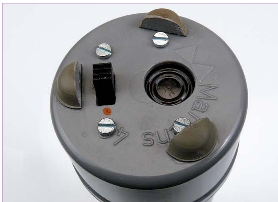
Figure 4. The on/off switch and a speaker are fitted in the end cap.
